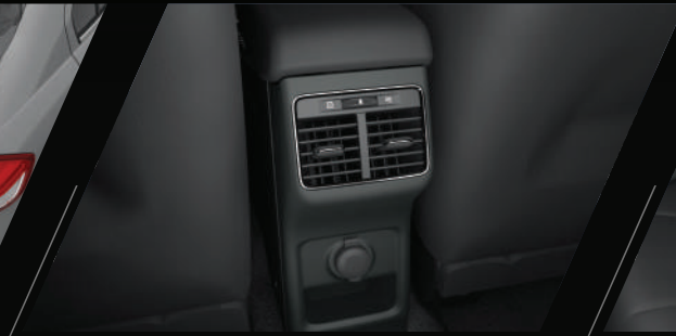
Rear AC vents and 12V accessory socket.
