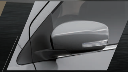
Electric side mirrors with turn signal lamps for added safety.
