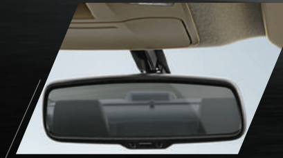
Automatic electrochromic rear view mirror.
