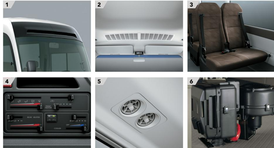
1. Large roof vents supply ample air for ventilation, both natural and fan assisted.
