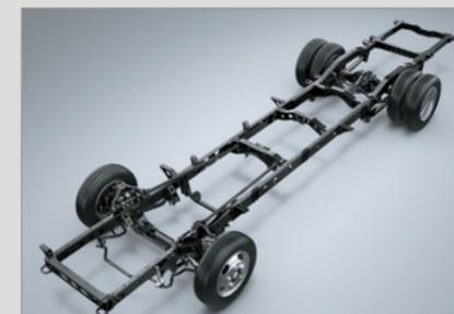
Extensive use of galvanised steel and deep, multi-layer paint coating protects the body from natural elements.
